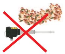
Material should not touch on the pedal. You should protection plate on the top.
