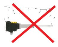
In case vapour splash cable potting points,insulation problem may cause.
