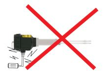
Excess current, to be drawn as a result of direct connection to motor, may burn relay of switch
