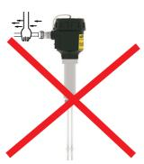
Do not pull the cable strongly, otherwise the characteristics might be changed.
