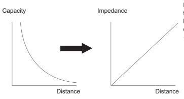
Excitation applied between 10 KHz...250 KHz based on length for all our models. ( $\omega$  =2xpxf) Linearity error that may be caused by conductivity component (R) effect is prevented by electronic circuit design and mechanical design. Reduced to a level lower than 1ppm, acceptable as zero.
