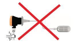
Do not pull the cable strongly, otherwise the characteristics might be changed.
