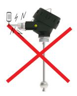
Excess current, to be drawn as a result of direct connection to motor, may burn relay of switch
