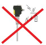
Excess current, to be drawn as a result of direct connection to motor, may burn relay of switch
