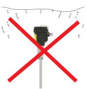
In case vapour splash cable potting points,insulation problem may cause.
