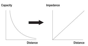
Excitation applied between 10 KHz...250 KHz based on length for all our models. ( $\omega$ =2 x p x f) Linearity error that may be caused by conductivity component (R) effect is prevented by electronic circuit design and mechanical design. Reduced to a level lower than 1ppm, acceptable as zero.
