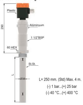
**ECAS 204 Partly Insulated Rope Conductive Tank**
