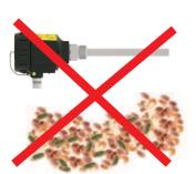
No material should come on the probe. You should put a guard plate on the top.
