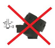
Do not pull the cable strongly, otherwise the characteristics might be changed.
