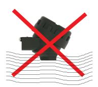
In case vapour splash cable potting points, insulation problem may cause.
