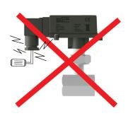
Excess current , to be drawn as a result of direct connection to motor, may burn relay of switch
