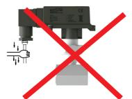
Do not pull the cable strongly, otherwise the characteristics might be changed.
