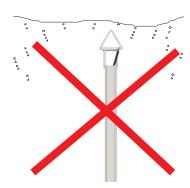
In case vapour splash cable potting points,insulation problem may cause.
