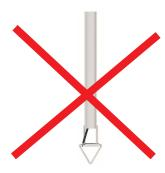
Do not remove the float from connection part. Because its pin might be damaged.
