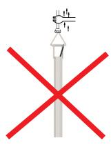
Do not pull the cable strongly, otherwise the characteristics might be changed.
